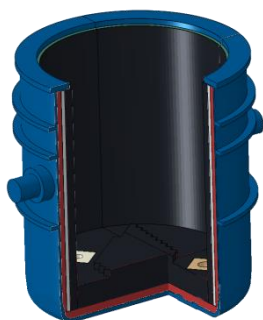
Fig. 1. Finite element model of a ladle
