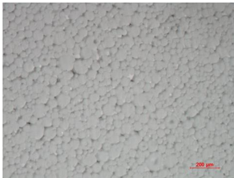
Fig. 1. MARTODIX KM-96 ALBEMARLE green bodies surface formed at 4 MPa.
